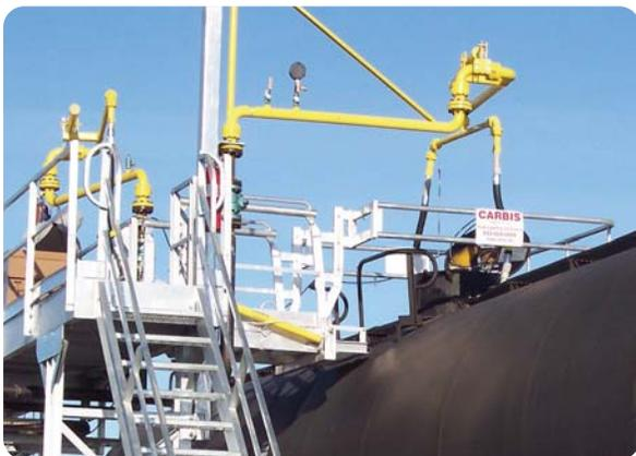
There are several arm designs that can be tailored to specific needs. Top loading arms include single arm fixed reach, scissor type, supported boom and unsupported boom. Bottom loading arms, which are the preference in the industry, have similar designs including an unsupported boom, A-frame, A-frame spring balanced and counterweighted. Marine loading arms load/unload barges and carriers.
