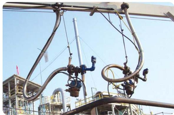
Most hose types can be created with reflex construction. A helix wire is often used as hose reinforcement but once the wire is bent or crushed enough to flatten or kink the hose wall, the wire becomes permanently damaged. A reflex hose on the other hand, bounces back to regain its shape and performance. A thick rubber filler block divides separate groups of wire reinforcement to keep this hose working under the cruelest conditions.<sup>3</sup>
