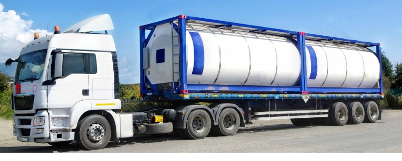
Lately, some companies have been adding elements to ISO container frames that create additional configuration issues. Extensions to the middle of the crossbar, for example, could add 12" to the frame, making the frame unstackable. Companies in the U.S. that send containers out of the country may also have to accommodate configurations and foreign standards that differ from those set by the ISO.
