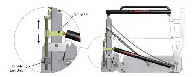
Adjustment to the spring counterbalance system may be required to change the amount of force necessary for the return of the gangway to the stored position. The springs are set at the factory for the gangway weight and any options that might have been purchased. These could include a seatainer end tread and/or a cage. It is necessary for all purchased options to be installed prior to use for the springs to properly function.
