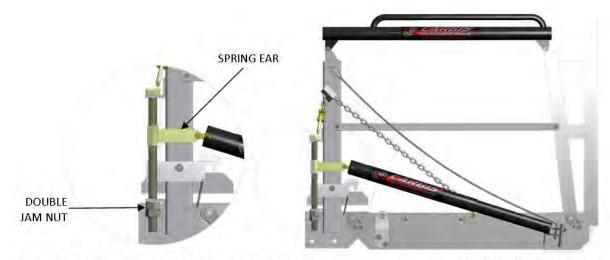
Adjustment to the spring counterbalance system may be required to change the amount of force necessary for the return of the gangway to the stored position. The springs are set at the factory for the gangway weight and any options that might have been purchased. These could include a seatainer end tread and/or a cage. It is necessary for all purchased options to be installed prior to use for the springs to properly function.
